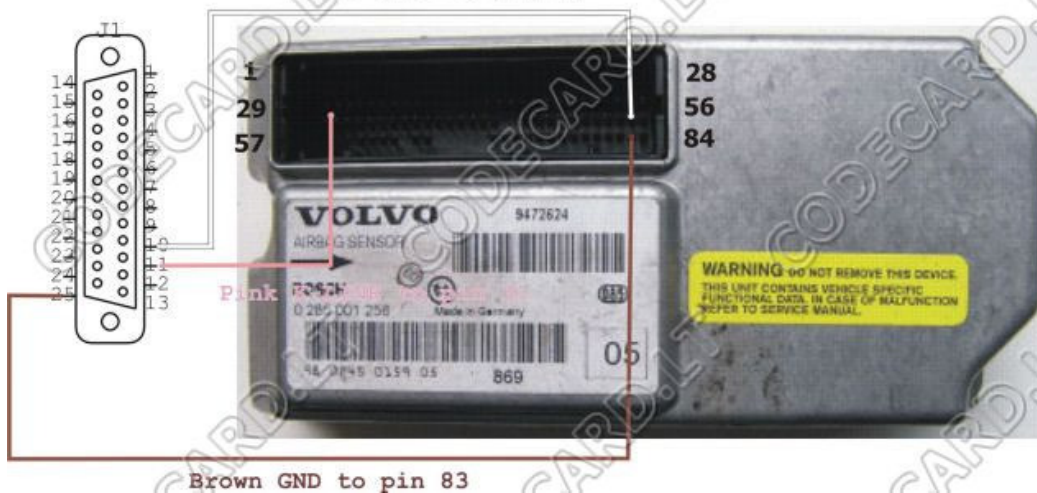
A15 cable connection to Volvo airbag sensor
